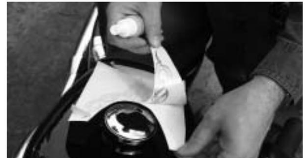
Release the graphic from the base by peeling backwards away from itself. Hold onto the backing paper as you do this. Notice that I have the spray bottle of Application Fluid in my hand for the next step.
