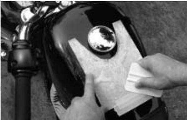
Lay the decal down and begin to squeegee it to the surface of the bike in a sweeping motion from the hinge, upward and outward with strong pressure.
