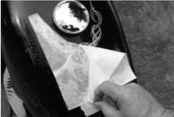
Begin removing the premask application tape by pulling it directly back against itself at 180° angle.
