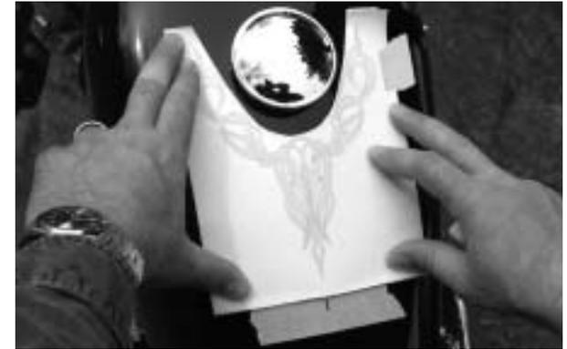
Position the graphic where you want it to be on the bike. Tape it in position if you need to. Take your time at this phase - where you position the decal is where it will end up. You can measure from the edges of the gas cap to make sure the decal is centered.
