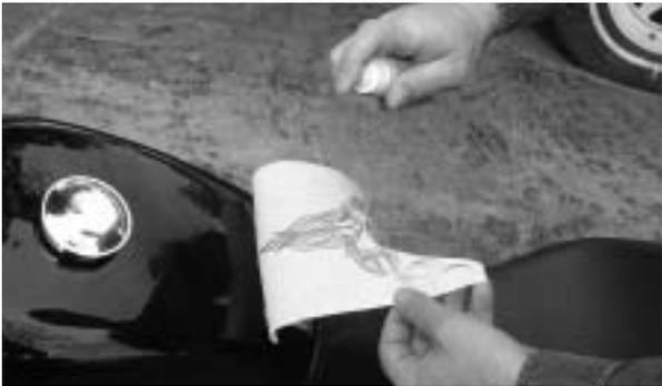
Holding decal away from motorcycle, spray liberally with Application Fluid (Green Label) on both the surface of the bike and the decal. This is important to prevent a haze under the decal.
