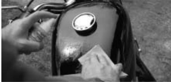
Begin by preparing the surface of the motorcycle to be decorated by spraying liberally with Preparation Fluid (Orange Label) and wiping vigorously with one of the blue lint-free towels supplied with the kit. Prepare all the surfaces which you intend to apply decals to at the same time. If you wax your bike frequently or have waxed it recently, it is also necessary to clean it thoroughly with wax and grease remover such as Prep-Sol available at any auto supply store.
