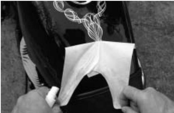
Continue pulling tape back to expose the entire decal. After removing the application tape completely, you can use the backing paper you saved earlier to burnish any
