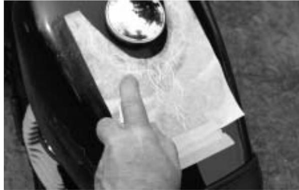
Spray the face of the decal with more Application Fluid. This helps release the adhesive from the decal and makes removal of the premask tape easier.
